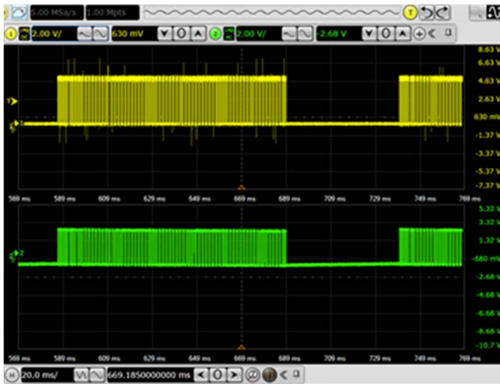
Figure 12. Emitted and received baseband waveforms.
